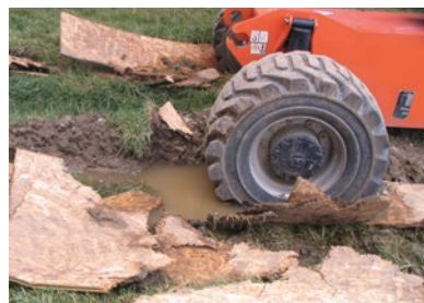
Plywood cracks under pressure
